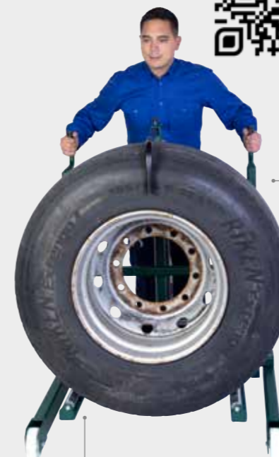
Rollers fitted with ball bearings easy for rotation and positioning of wheels.
