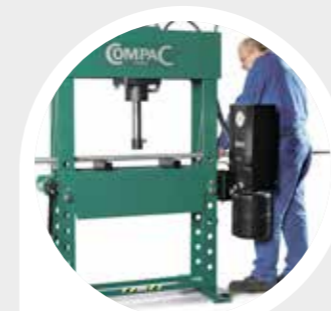
A 90° hinged pump unit enables easier insertion of longer work-pieces.
