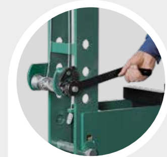
Fast and safe adjustment of the press table height, using a braked winch.
